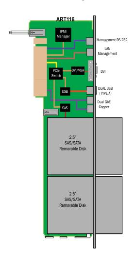
FIGURE 1. ART116 Functional Block Diagram
